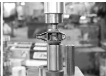
2. Gently press out the existing trunion using a ½ in. driver, being careful not to damage the rocker body. During the press out make sure that the die, driver and rocker arm remain straight. The factory trunion will unseat and come out relatively easily.
