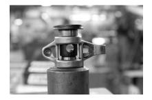
6. Drop in the trunion. Set the other bearing on top as flat as possible. Set 1 of the washers included with the kit on top of it, again letters facing outward. Press against washer so it slides around the trunion. Press only until light pressure is felt, this will start the top bearing install, ensuring everything stays lined up.
